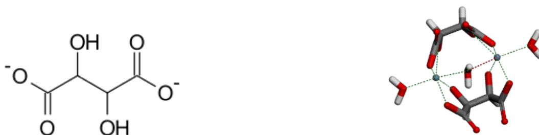
Figure 6 – The chemical formula for tartrate and a 3-D impression of a complexation product of tartrate with iron and water
