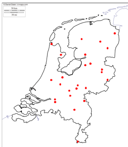
Figure 4 – Cyanide contaminated locations in the Netherlands because of de-icing salt storage in the period 2002 to 2012 (red dots).
